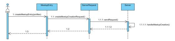
In this sequence, a meetup is first being made. A meetup entry will be made with the profiles of the matched users, and then placed onto the database, along with a list of the users. This second list will only ever be added to, and will be used for profile history.
