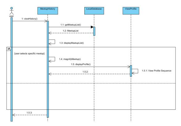
The View Meetup History sequence has minimized contact with the server, due to the method we have chosen to store meetups, outlined in Leave Meetup (app). The LocalDatabase will return a list of past meetups, and display them. A user will be able to magnify a meetup to see more detail about it, and view user's profiles that were part of the meetup. The View Profile sequence takes place at this time, and this is the only point in which this sequence has server contact.
