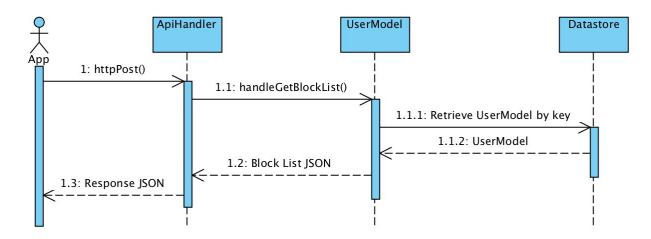
When the user wants to view their block list, the server retrieves the user's data from the database through the use of the user key provided when the user logged in. The block list containing usernames of blocked users is returned back to the app.
