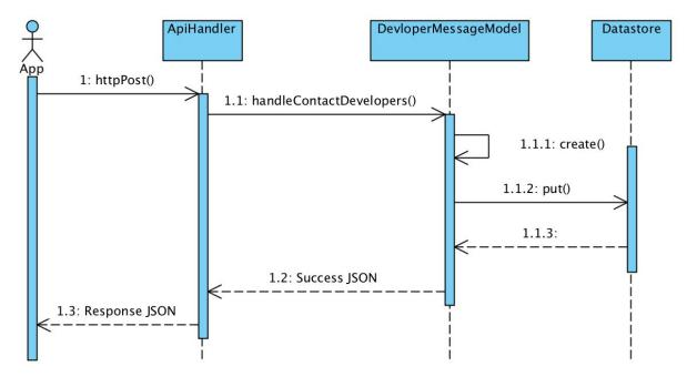
When the user desires to send a message to the developers of the app, the app sends the user key and the message to the server. The server receives this request and creates a new developer message that is stored in the datastore. The server then responds indicating the request has been successfully sent.
