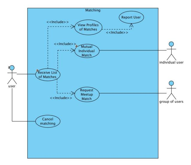
The **Meetup Matching** use case encompasses the activities a user can do during a search for a meetup. These are limited to cancelling the searching/matching service, viewing profile of potential matches, as well as toggling willingness to match with a user or meetup.
