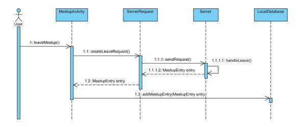
In this sequence, a user leaves a meetup they are currently in. A request will be made to the server to remove the user from the meetup. The server will handle the removal of the user, and return a Meetup Entry. This Meetup Entry consists of all previous users in the meetup, which is stored separately than the list of active users. The Meetup Entry will then be placed on the phone or device's local database, as part of the user's meetup history.
