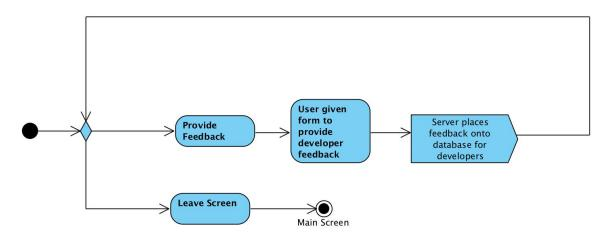
The user can choose to provide feedback on the app and is prompted to enter their feedback into a text form. The feedback is sent to the server when the user finishes filling out the form.
