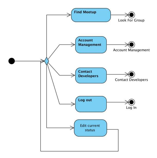
From the main screen, the user can choose to start searching for a meetup, manage their account, contact the developers, or log out. A potential feature is the ability to edit a user's status, should statuses be implemented.
