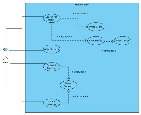
The **In A Meetup** Use Case encompasses activities a user can perform whilst in a group. These are limited to accepting new users, viewing users currently in one's group, locating these users, leaving meetups, and inviting friends to the meetup. We hope to implement the ability for meetups to search for individual users or other meetups, but this is currently a possible feature, not a required one.
