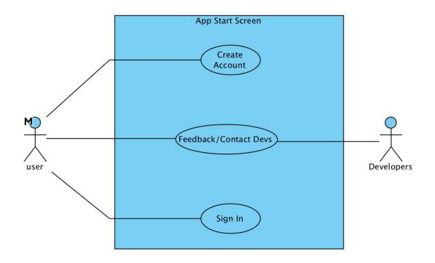
The Log-In Use Case encompasses activities a user can perform before logging into the application or creating an account. These are limited in scope to creating accounts and contacting the developers with feedback, as well as signing in. Recovering accounts will be unnecessary with our method of logging in, and reactivating accounts, if implemented, will occur automatically upon sign in.
