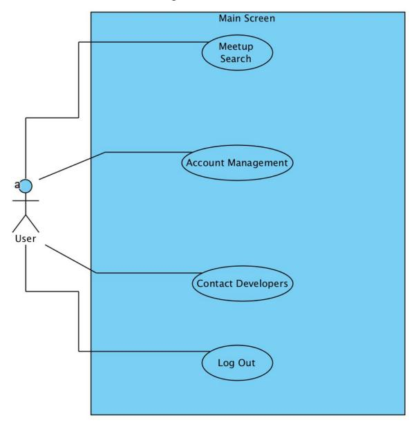
The **Main Screen** use case outlines what a user will be doing when on the primary screen of the application. These cases include searching for a meetup, managing one's account, contacting the developers with feedback, and logging out of the application. If time permits, the ability to edit a user's status will be available in this use case as well.
